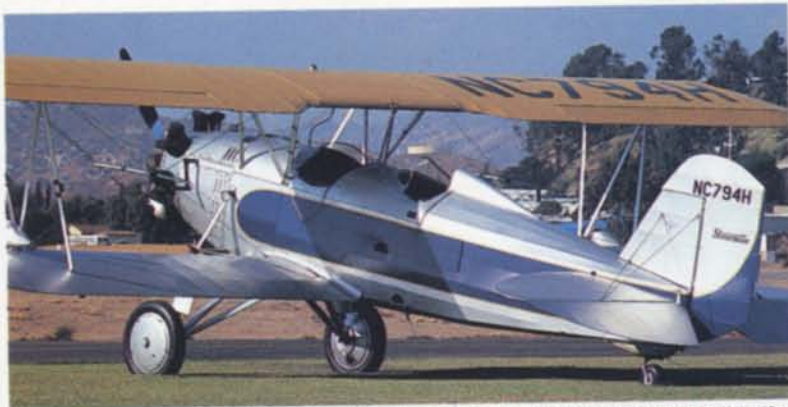
The C3R received a number of modifications over the previous C3B, including the pilot's headrest. Here, the crank for the inertia starter can be seen.
