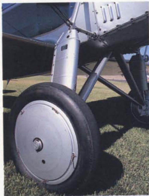
Left: the C3R's long-stroke landing gear was designed for rough, sod fields. The wire-spoked wheels are covered with aluminum that is secured with rawhide ties. Right: the streamlined landing lights on each wing helped the pilot find the runway and avoid cows during night landings.
