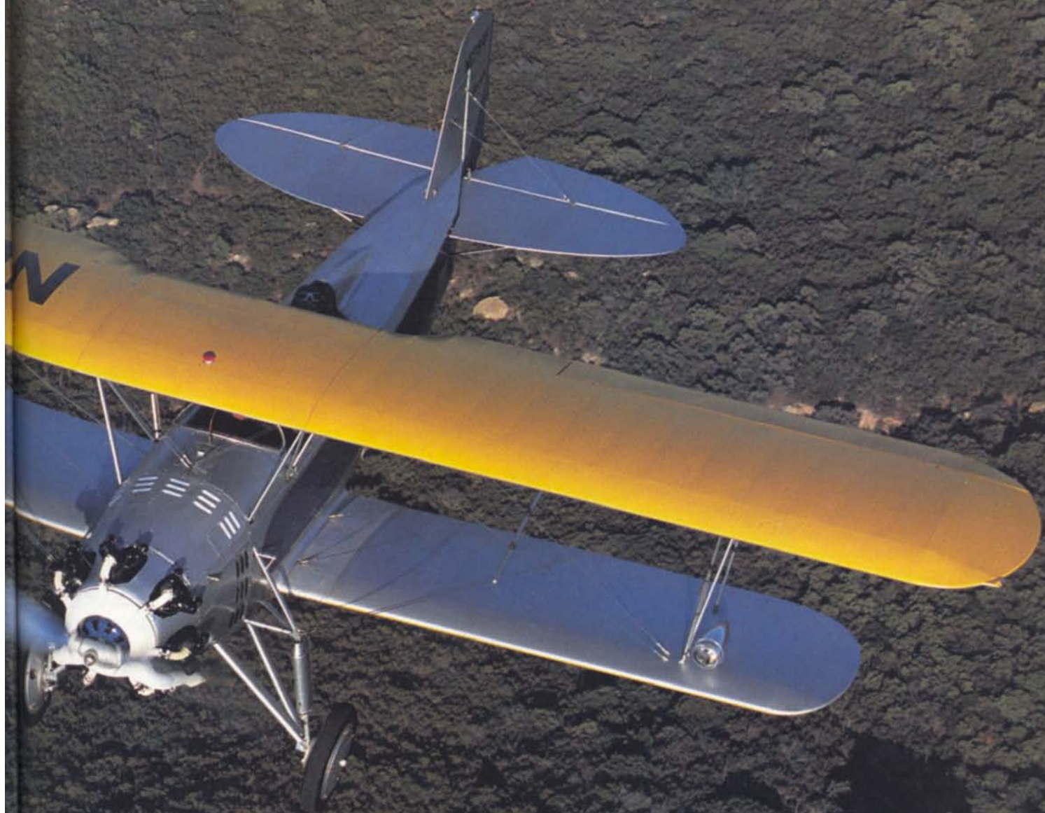
The 225hp Wright J-6-7 moves the big biplane along at 105mph which, in 1930, gave the owner/pilot airline performance and utility.
