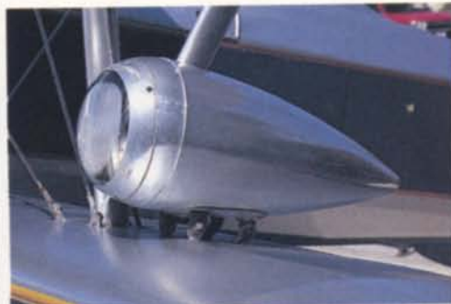
Left: the C3R's long-stroke landing gear was designed for rough, sod fields. The wire-spoked wheels are covered with aluminum that is secured with rawhide ties. Right: the streamlined landing lights on each wing helped the pilot find the runway and avoid cows during night landings.
